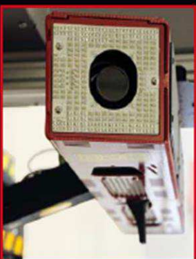
Laser distance sensor for ift and wheel search
